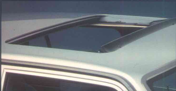
In addition to conventional opening it can also be raised at the back for totally draught-free ventilation.
