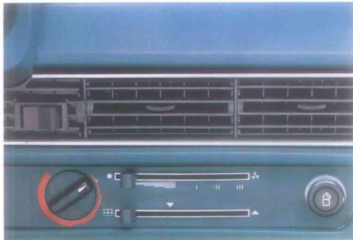
Flow-through ventilation distributes the air throughout the passenger compartment.
