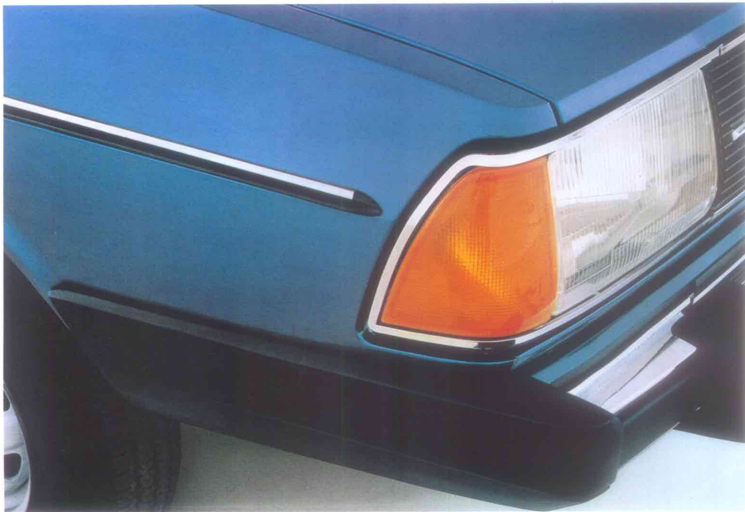
Bumper side extensions for added protection. Adjustable wide beam halogen headlights.
