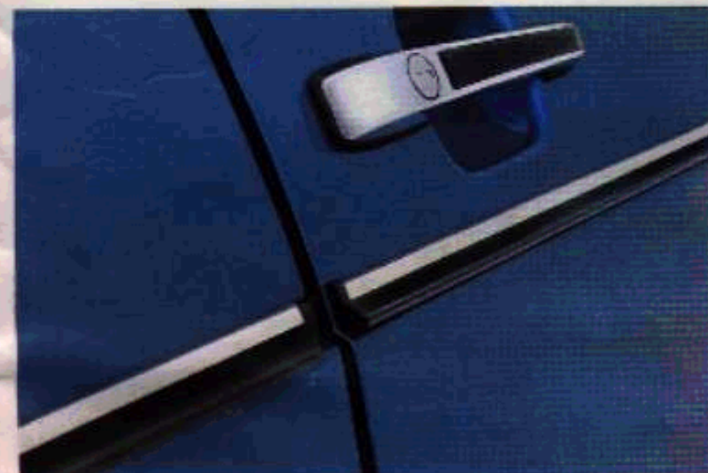
The trim around the car's waistline has a rubber strip to protect the paintwork.
