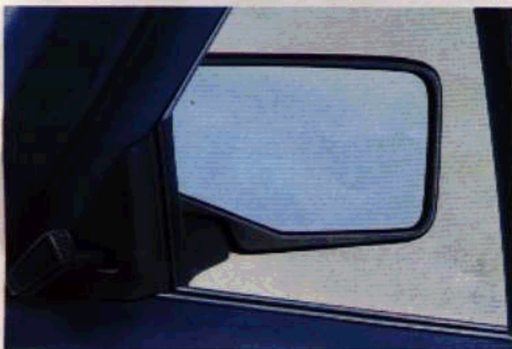
16 You can adjust the outside mirror from inside the car.
