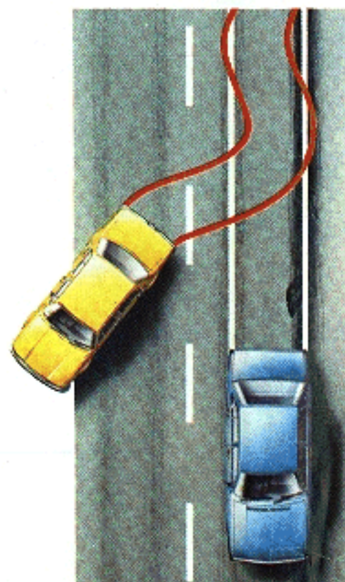
With oil on one side of the road, the Audi 100 with its steering stabilising and braking system stays straight on course. The car with a conventional braking system veers to one side.
