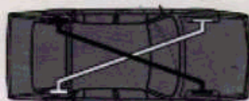
Even if one brake circuit fails, the braking pressure is evenly distributed.
