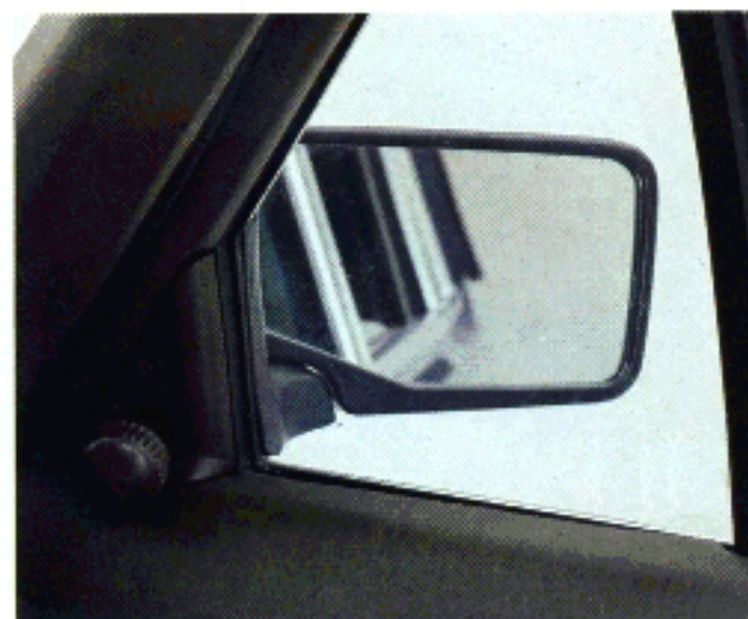
You can adjust the outside mirror from inside the car.
