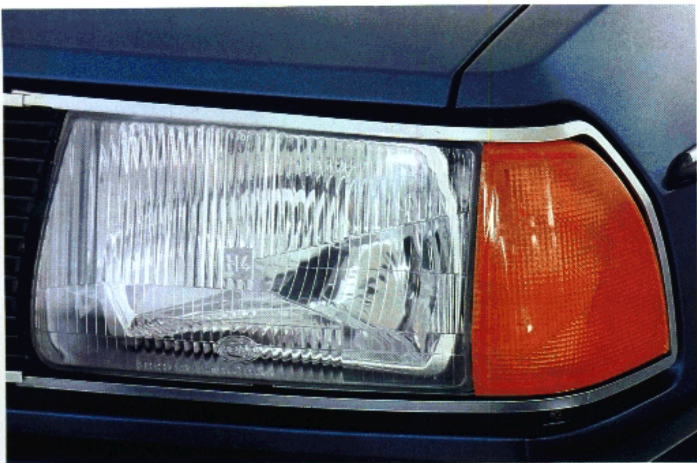
Adjustable wide beam halogen headlights.
