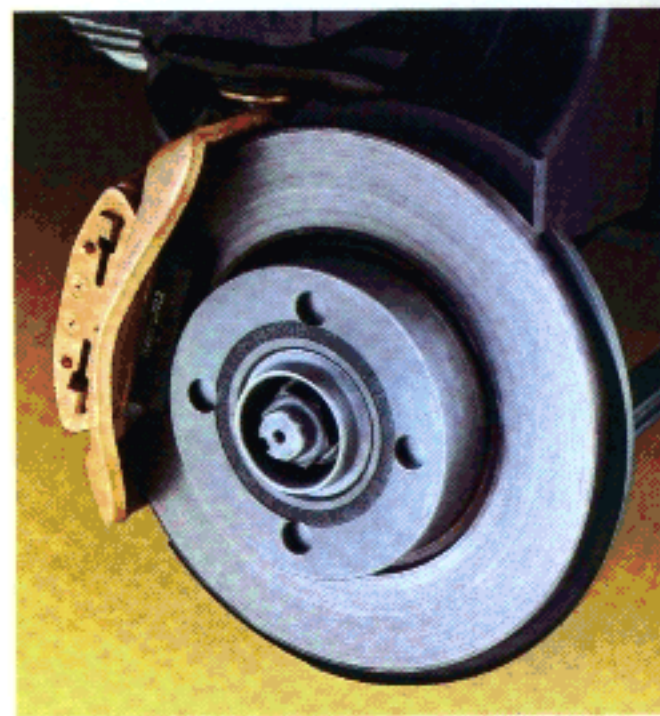
Large, floating caliper front discs.
