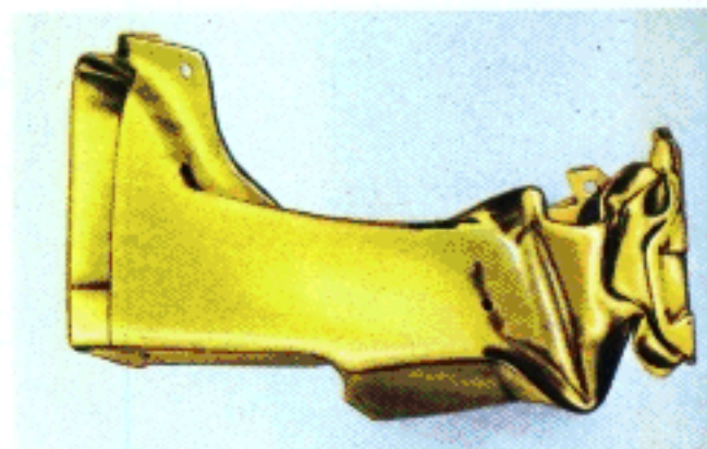
The front side members of the Audi 100 can resist a frontal impact of 40 mph.
